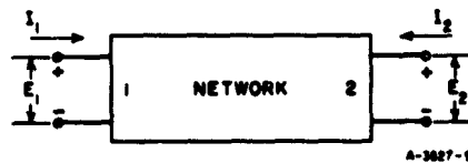
FIG. 2.05-1 DEFINITION OF CURRENTS AND VOLTAGES FOR TWO-PORT NETWORKS
