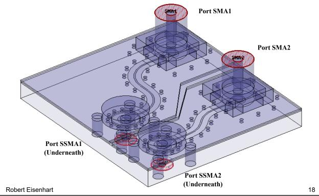
This example circuit will be used to demonstrate the performance of match at the connector ports and the isolation between the ports. Using stripline with side grounds (vias), lots of vias and a physical break in the grounds, we have two paths within one board.
