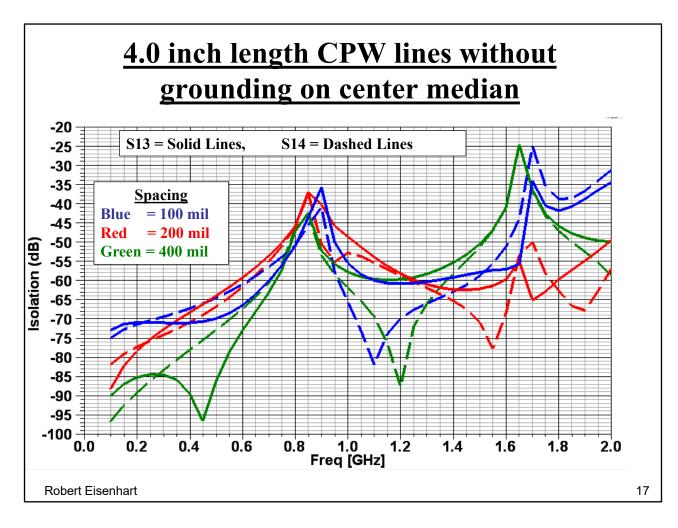
A special case is shown where the grounding strips (representing a perfect wall of vias) have been removed from the "ground" metalization between the lines. The coupling (worst isolation) is much stronger for all spacing's and is actually pretty independent of the spacing. This is no doubt due to the coupling beneath the "ground" strip as a parallel plate mode.
