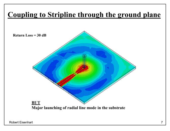
This has a good match (30 dB) at 1 GHz but all the input energy is not going to the port,
