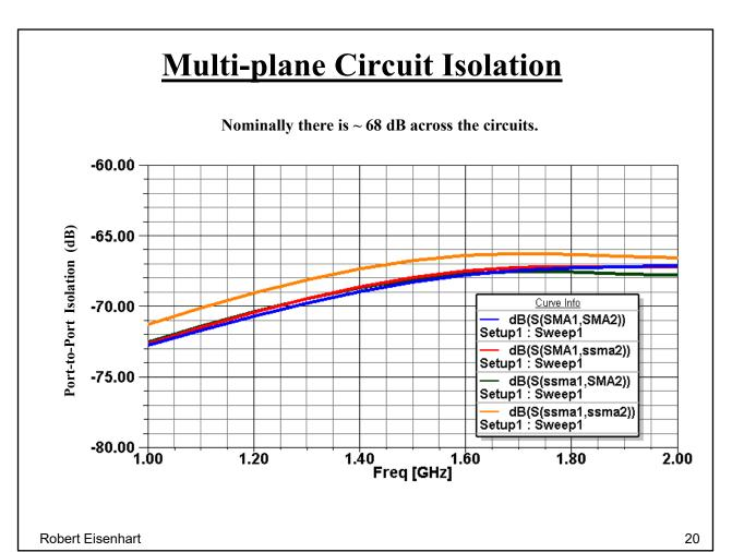
Isolation is fairly consistent, generally getting worse with frequency, as expected, however we desire <-100 dB isolation so we must determine how the energy is getting through.
