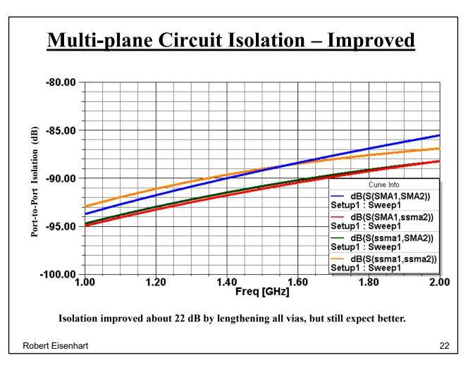
After better isolation around the SMAs, the isolation has significant improvement of 22 dB. Now to deal with suspected leakage above the board between connectors.
