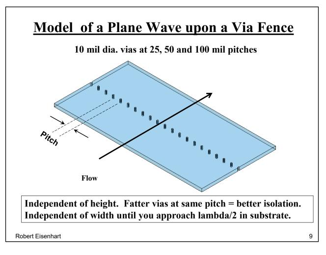
Parallel plate mode between two ground planes. Can be modeled on a single cell basis with a parameter of dia/pitch. This propagation is independent of the ground plane spacing and has no lower cutoff frequency. Let's look at incident radiation.
