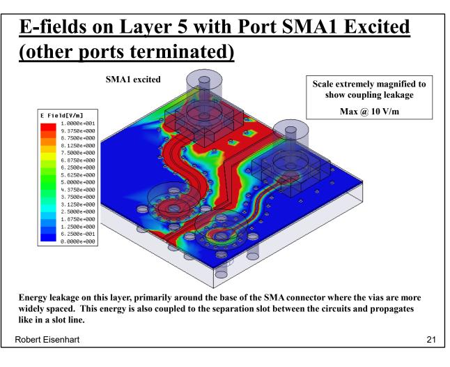
This is in the plane of the stripline center conductor. Leakage from the entry coax launcher, coupling to the break in the ground planes and propagating like a slot transmission line.
