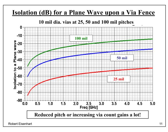
The "shorting effect" of the vias is related to how much of the opening exists, normalized to wavelength.
