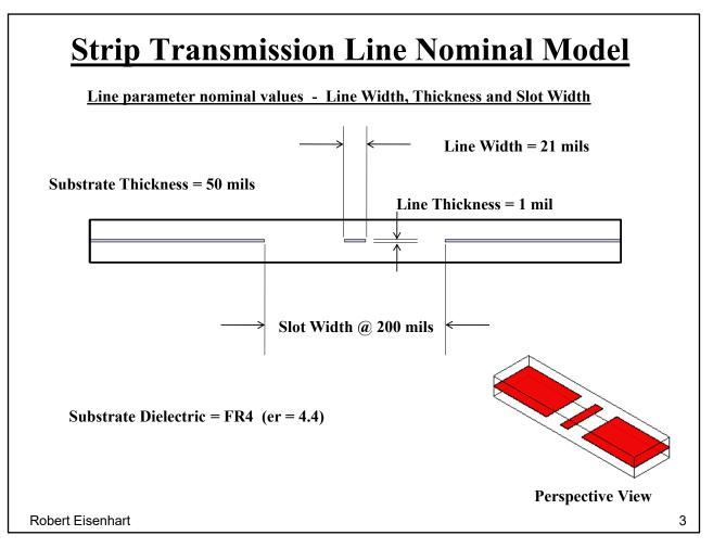
The top and bottom surfaces are ground and tied to the co-planar grounds on the sides.
