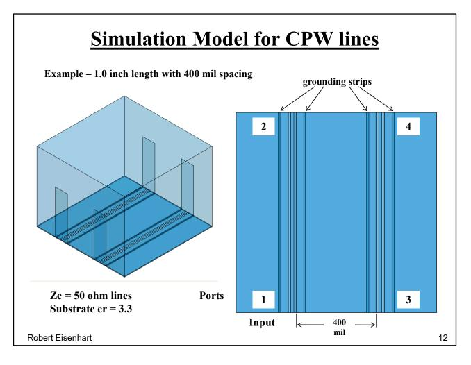
Looking for the isolation (or coupling) between two CPW transmission lines running parallel to one another with varied spacing at different lengths. This shows the general layout for a model using a 400 mil spacing (width of the center ground) between the lines at 1.0 inch in length.
