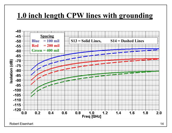
Here we see the coupling at 1 inch length lines. Note that the reverse coupling (S13) is slightly stronger than the forward coupling (S14).
