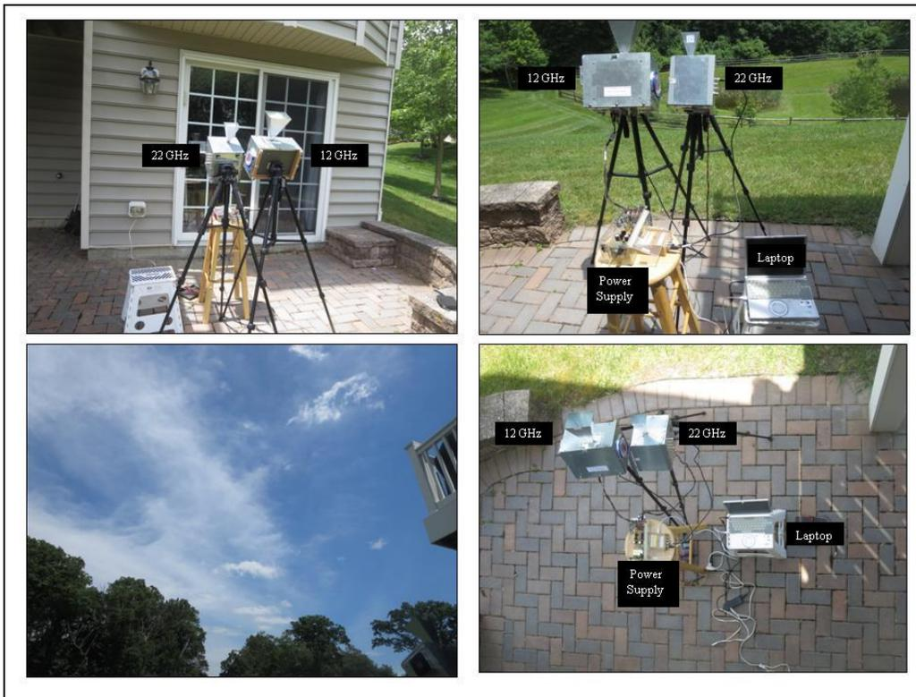
Figure 47. Top pictures show the radiometers mounted on tripods viewing the sky from my patio on June 15, 2020. The bottom-left shows the clouds seen while the bottom-right shows the setup.
