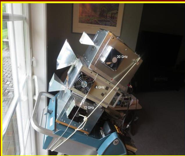
Homemade Radiometers at 4, 12 and 20 GHz
