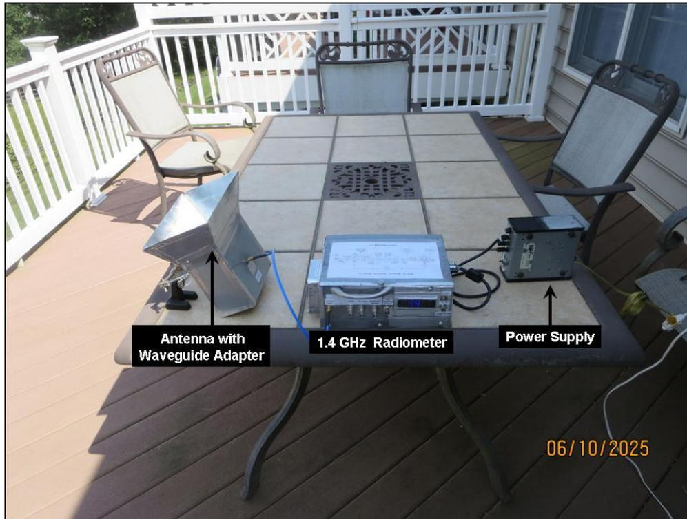
Figure A22-7. The radiometer's antenna is shown viewing cold space from my upper patio deck. The antenna is tilted away from the back side of my house to reduce ground - reflected radiation from entering the antenna sidelobes. For this antenna position the radiometer output is at its lowest value of -9.73 volts. Also, the radiometer offset is set to zero when the antenna views my body at 310 K. Therefore, the calibration equation is  $T_b(K) = 310 + 31.5 V$  (Volts).
