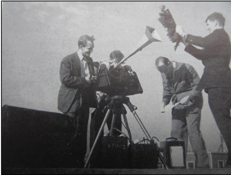
Figure 41 - Tipping curve absorption measurements by Dr. Robert Dicke along with his associates. Starting on the Left is E. Beringer, R. Kyhl, A. Vane and R. Dicke. It shows Dicke holding up a “shaggy dog” absorber in front of one of his radiometers while a chart recorder on the ground plots the measurements. This picture is in the book “Five Years at the Radiation Laboratory, MIT, by C. Newton, T.E. Peterson and N. J. Perkins (Eds.),” *The Andover Press, Ltd.*, 205 pgs., 1946.
