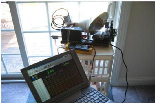
Figure A1-3 - 12 GHz Total Power radiometer measuring water droplets from a garden sprinkler.
